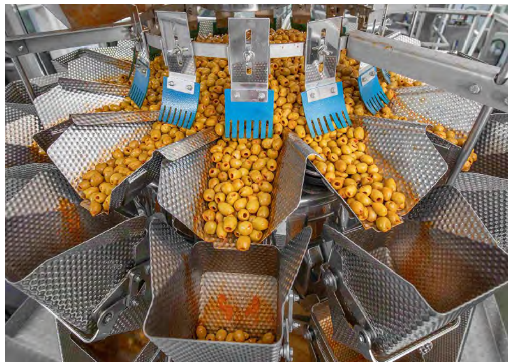
Top of CCW-RVE multihead weigher with orange olives
